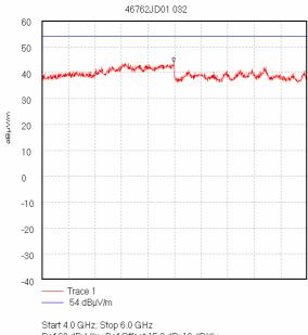
Start 4.0 GHz; Stop 6.0 GHz Ref 60 dBµV/m; Ref Offset 15.8 dB; 10 dB/div RBW 1.0 MHz; VBW 1.0 MHz; Att 0 dB; Swp 20.0 mS Peak 4.993 GHz, 43.78 dBµV/m Display Line: 54 dBµV/m; 09/12/2004 11:52:23
