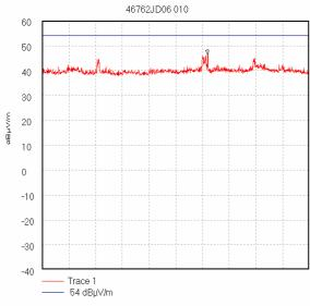
Start 1.0 GHz; Stop 2.0 GHz Ref 60 dBµV/m; Ref Offset 0.0 dB; 10 dB/div RBW 1000.0 kHz; VBW 1.0 MHz; Att 0 dB; Swp 20.0 mS Peak 1.62 GHz, 46.32 dBµV/m Display Line: 54 dBµV/m; ; Limit Test Passed Transducer Factors: 1 to 2
