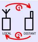
REQ\_READ\_REMOTE\_RSSI : request the RSSI level of the signal 1. (i.e. the RSSI level on signal 1 reception by the distant equipment)
