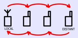
Remark: in the case of a REQ\_SEND\_FRAME request, the routing of the response towards the local equipment is not automatic. It must be configured by the distant host (user application).
