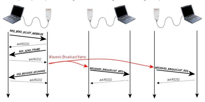
Reception of the END\_MESSAGE\_EXCHANGE command depends on the activation of the EXCHANGE\_STATUS parameter (0x0E). This command allows the equipment host to know exactly the moment from which WaveCard is available for communication RS232.
