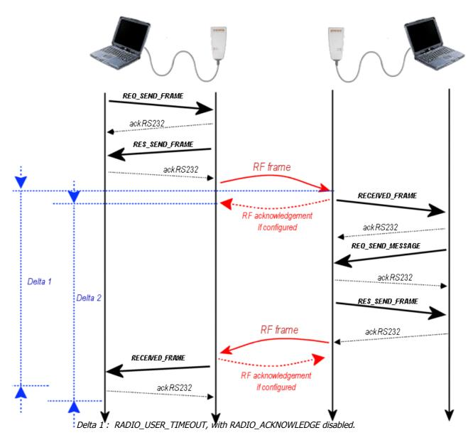
Delta 2: RADIO\_USER\_TIMEOUT, with RADIO\_ACKNOWLEDGE enabled.
