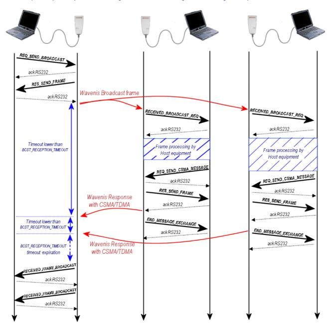
Reception of the END\_MESSAGE\_EXCHANGE command depends on the activation of the EXCHANGE\_STATUS parameter (0x0E). This command allows the equipment host to know exactly the moment from which WaveCard is available for communication RS232.
