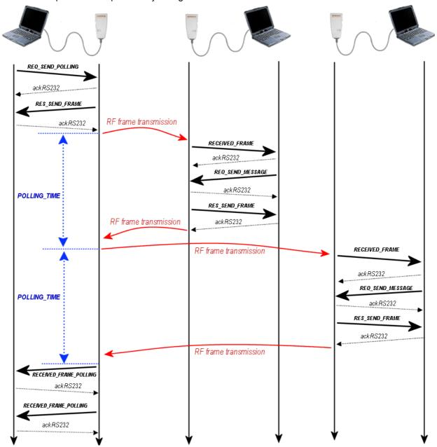
**POLLING\_TIME**: after transmitting the radio frame, a timeout is started (configured by POLLING\_TIME parameter); and if the equipment doesn't respond before the end of the timeout (1 second by default), then the transmitter send the same radio frame to the next distant equipment. However, if the previous distant equipment responded after this timeout; its response frame would be lost.
