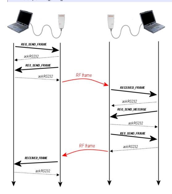
In this example, from the request transmitter side, the frame RECEIVED\_FRAME is the response associated to the request REQ\_SEND\_FRAME.
