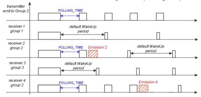
Synchronization allows a faster response of the modules (Since it don't use Long WakeUp) and optimize consumption.
