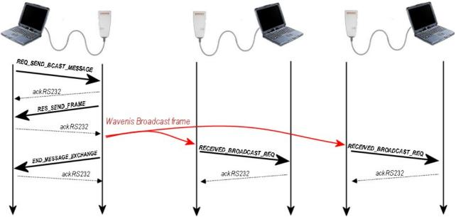
Reception of the END\_MESSAGE\_EXCHANGE command depends on the activation of the EXCHANGE\_STATUS parameter (0x0E). This command allows the equipment host to know exactly the moment from which WaveCard is available for communication RS232.
