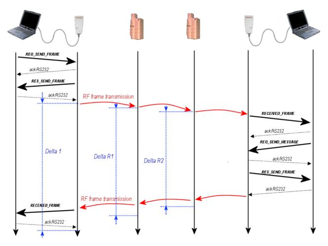
In the case of the Relaying mode, the time-out from the transmitter point of view is longer than in Point-to-point mode, because of the transit via the relays.
