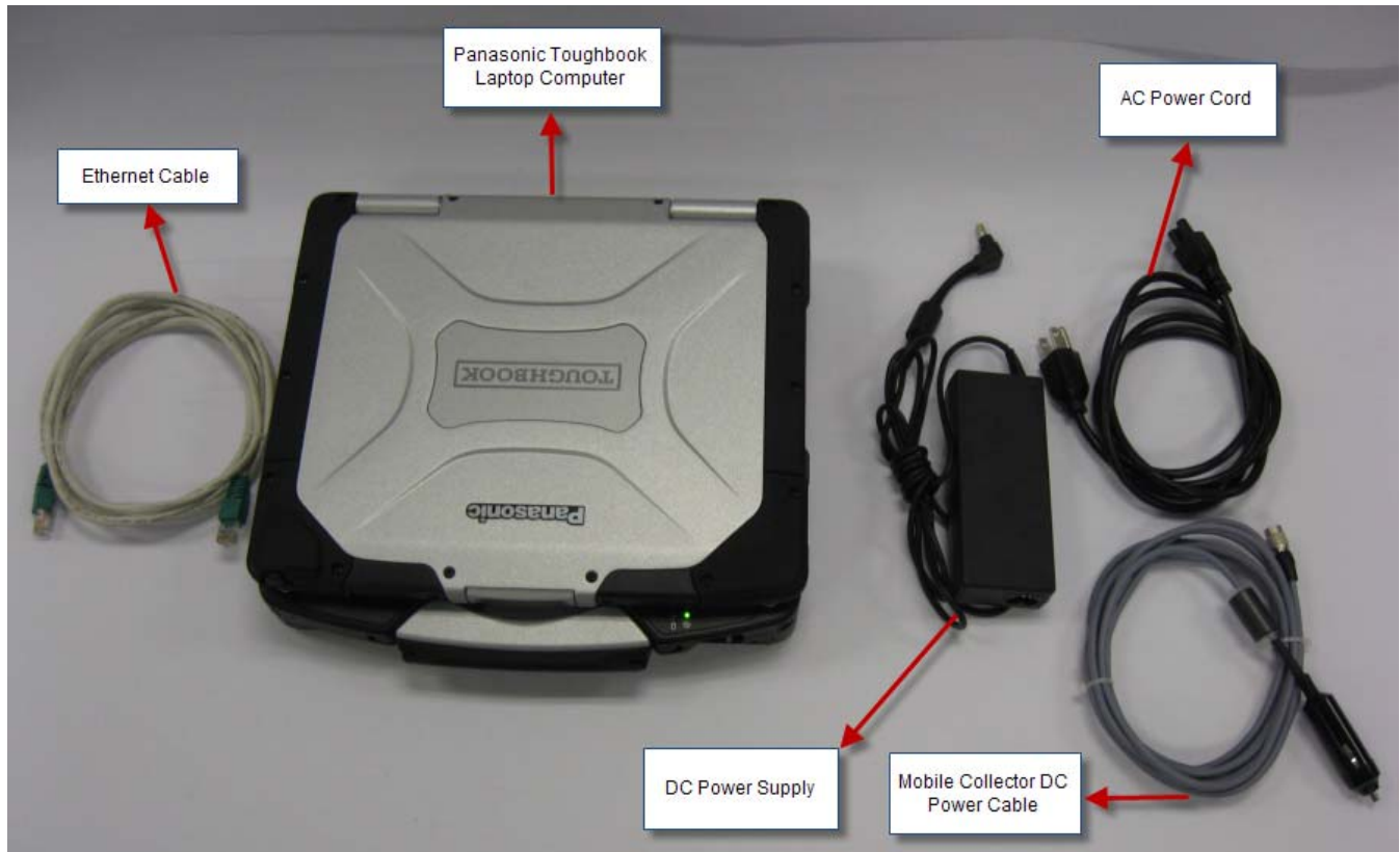
Figure 1: The evoDrive ruggedized notebook PC with included accessories
