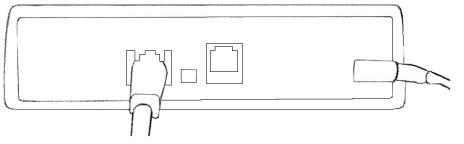
Insert Ethernet Cable Here Insert Power Supply Cable Here
