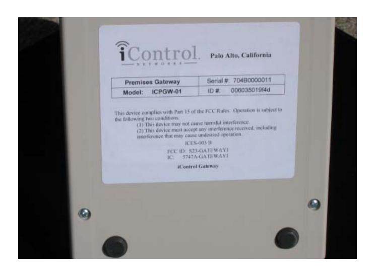
Label is located on the base of the device as shown above
