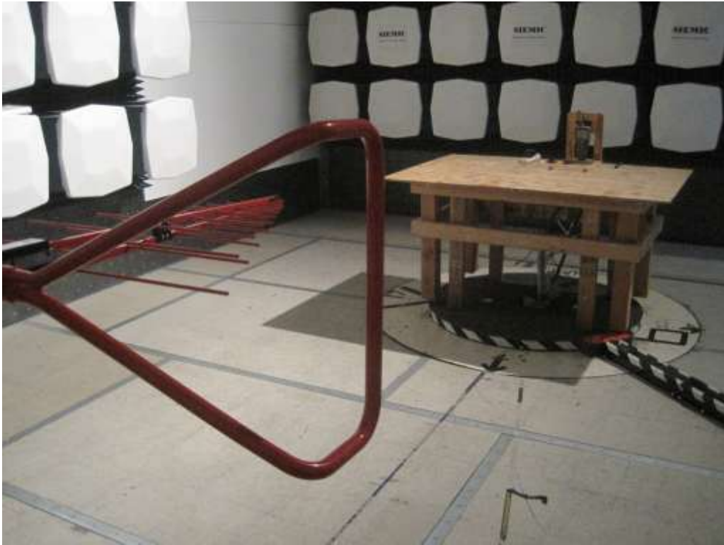
Radiated Emission below 1GHz (PHI 470) - Front View
