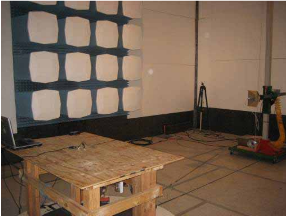
Radiated Emission above 1GHz-Handheld EUT
