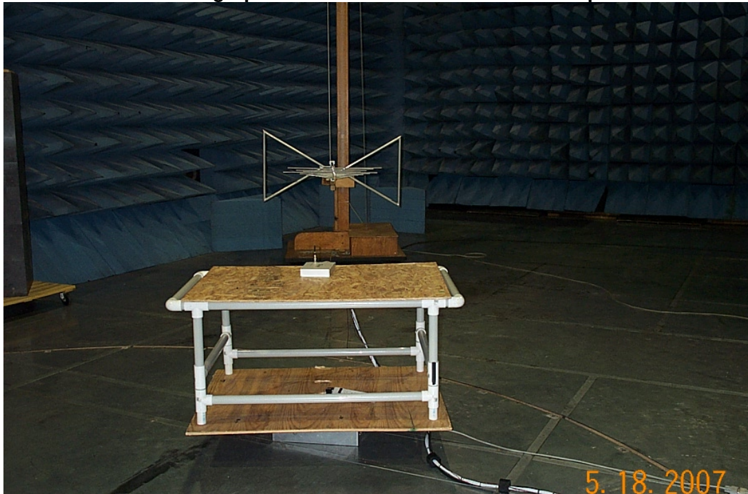
Photograph of Radiated Emissions Test Setup
