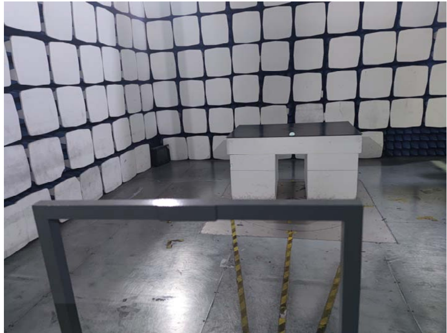
Radiation Emission Test Setup (Below 30MHz)
