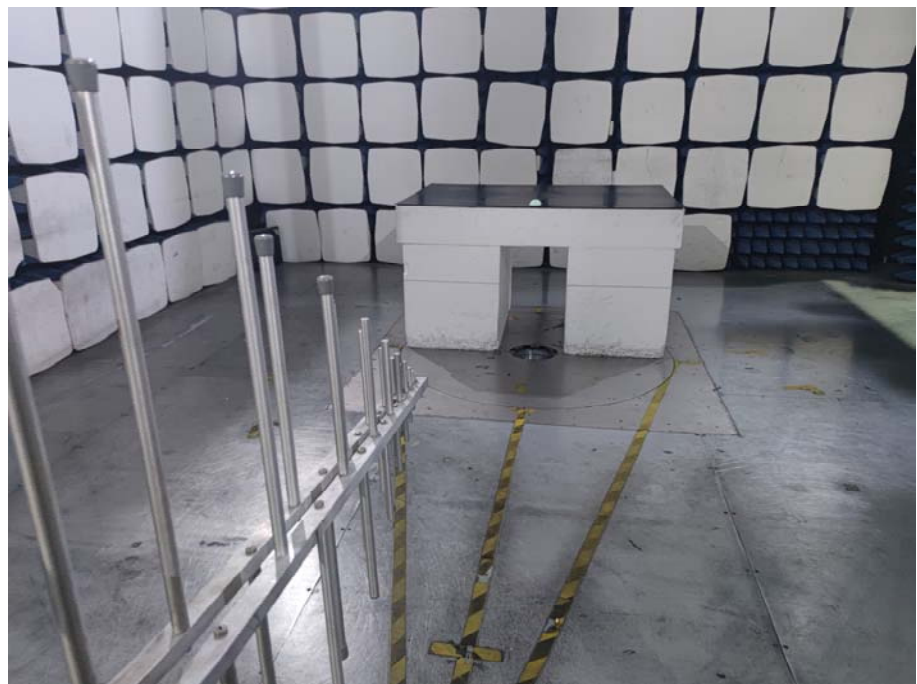
Radiation Emission Test Setup (30MHz to 1GHz)
