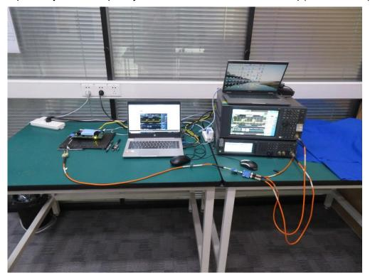
Description: Dynamic Frequency Selection Measurement Test Setup(Mesh Mode)
