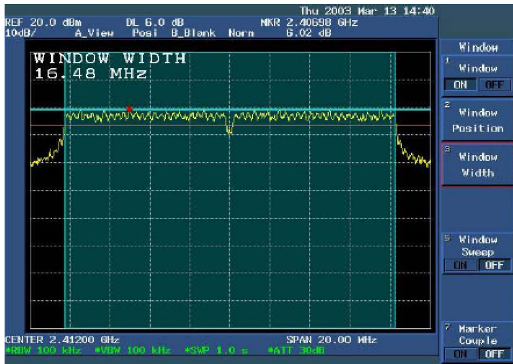
Plots of 6dB Bandwidth for 802.11g (15.247)
