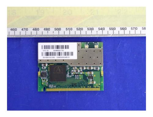
**EUT – Transceiver Component View without Shielding**
