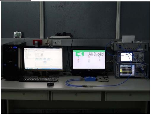
**DFS Set-up Photo: Master and Slave (UUT)**
