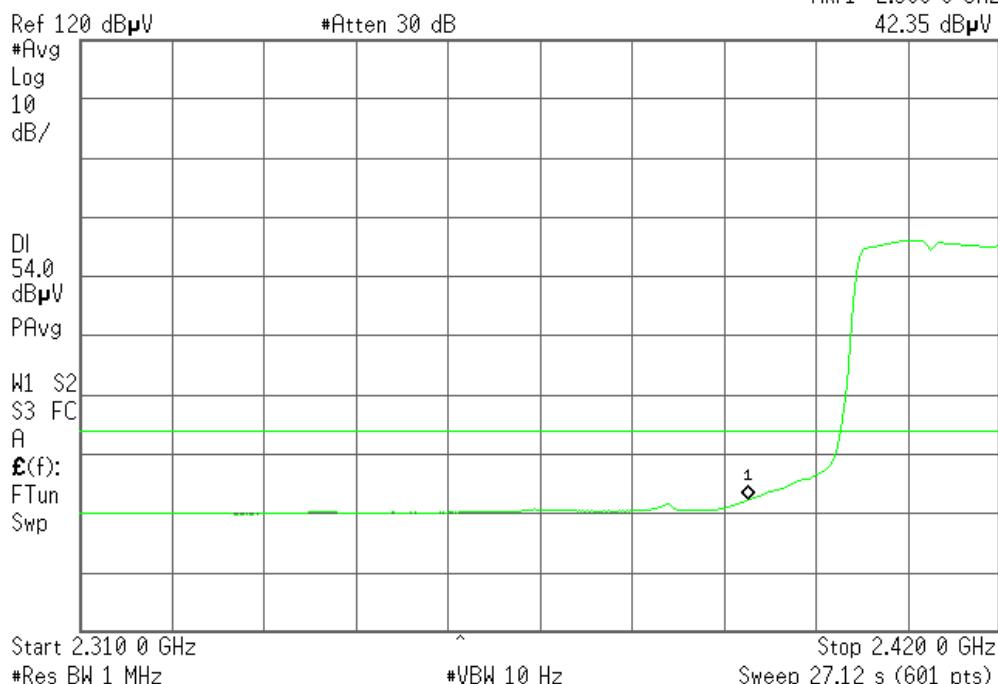
**Band Edges (IEEE 802.11n HT20 MHz mode/ CH High)****Detector mode: Peak**
