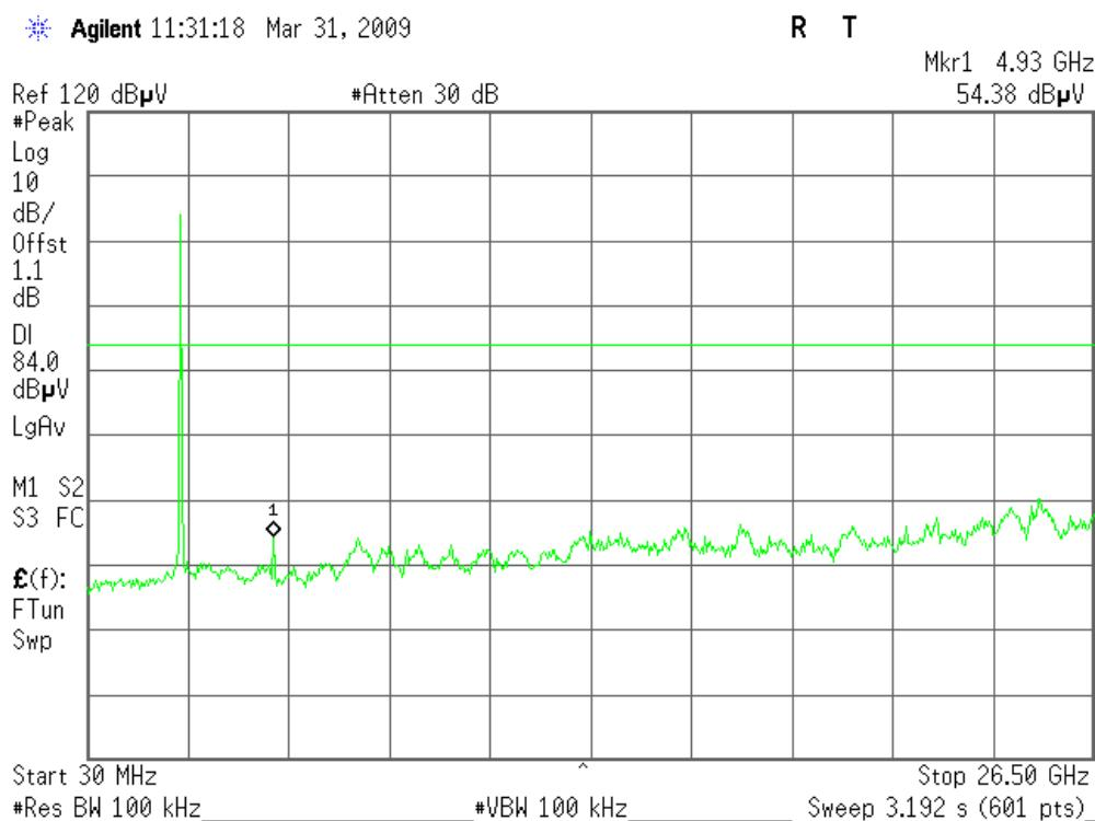
IEEE 802.11n HT20 MHz mode / CH Low**30MHz ~26.5GHz**
