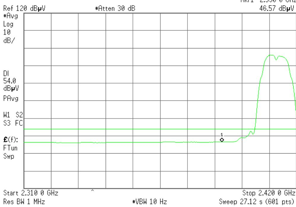
**Band Edges (IEEE 802.11b mode/ CH High)****Detector mode: Peak**
