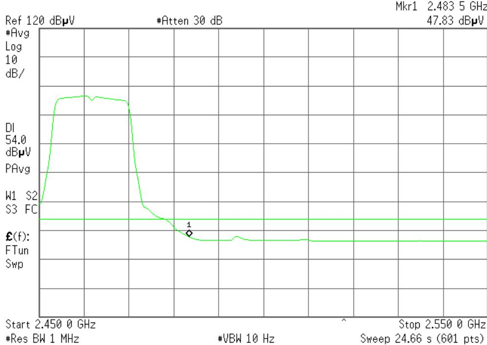
**Band Edges (IEEE 802.11n HT20 MHz mode / CH Low)****Detector mode: Peak**
