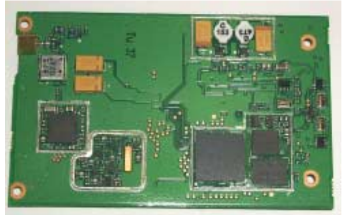
Photograph 9-4: Back side of module main board with shields removed.
