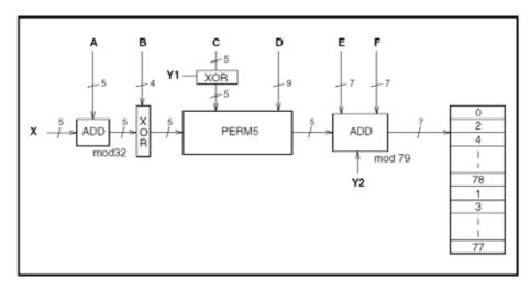
Due to the above flow, 32 hops are made into 5 ways. Then, the sign of the sign head 160 is formed. The remainder that is worked out by dividing with 79 is assigned to Hopping Channel.
