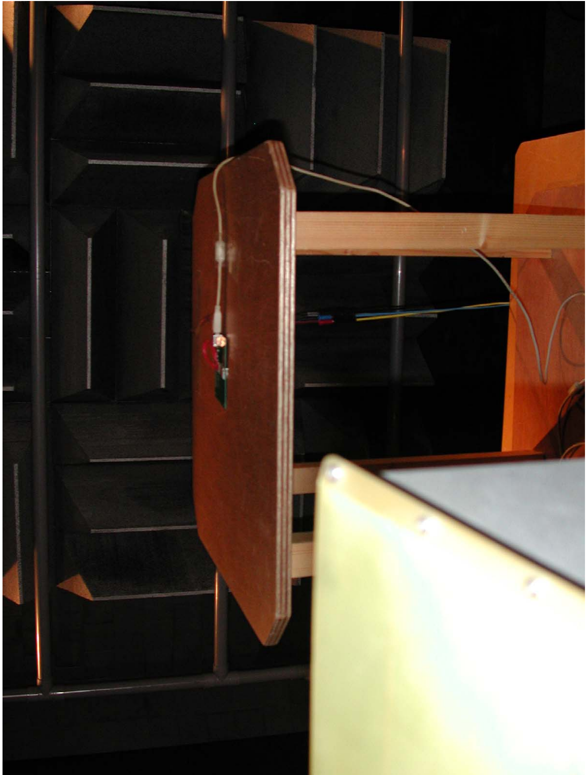
Photograph 2: Radiated measurements test setup > 1000 MHz
