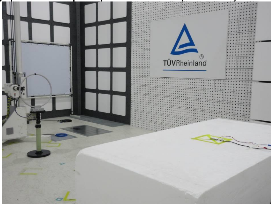
Photograph 4: Test Setup for Spurious Emissions (Back View 2)
