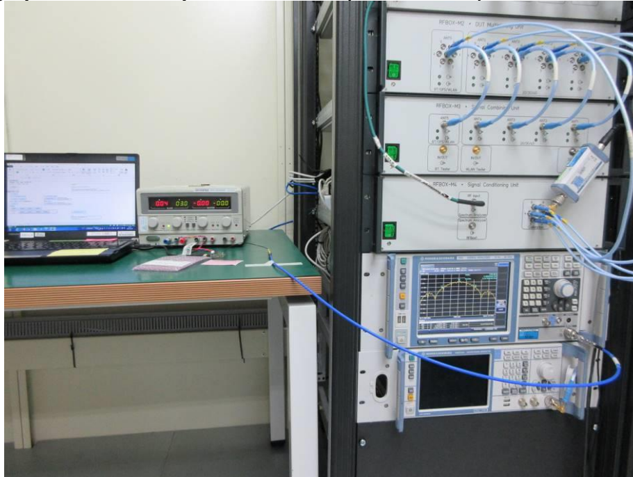
Photograph 11: Test Setup for Conducted (IEEE802.15.4)
