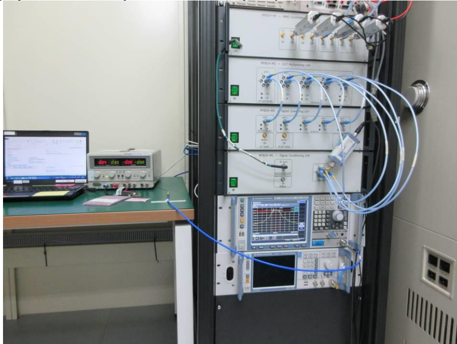
Photograph 9: Test Setup for Conducted (BLE)
