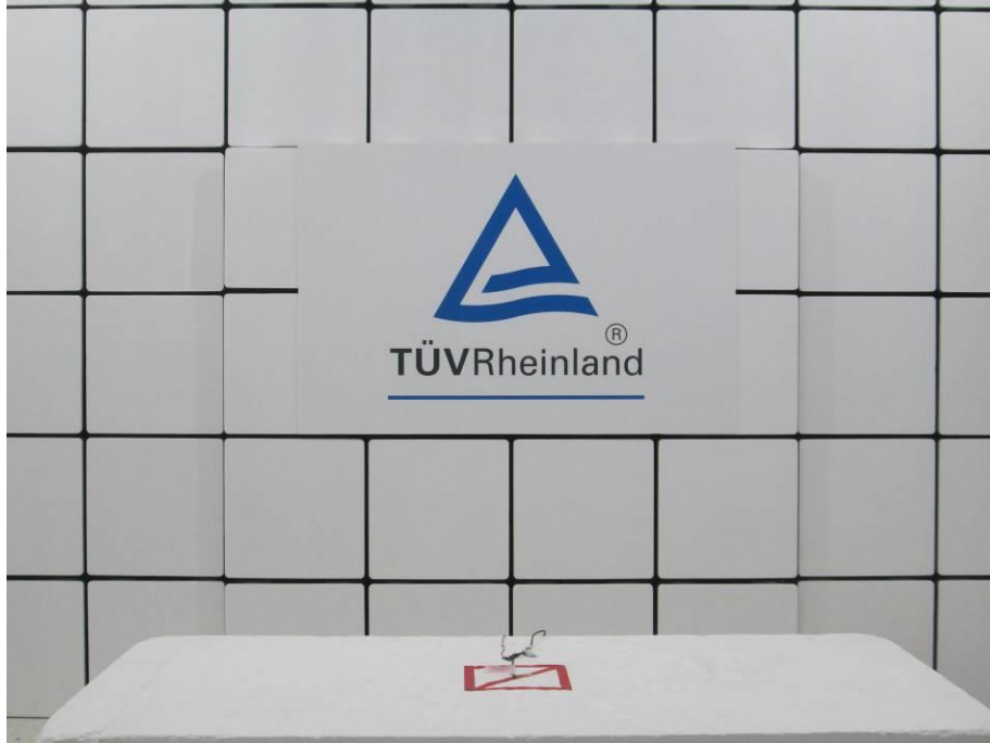
Photograph 1: Test Setup for Spurious Emissions (Front View 1)
