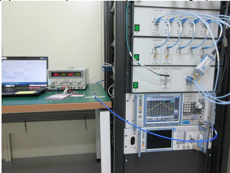
Photograph 10: Test Setup for Conducted (ANT & Nordic Original)
