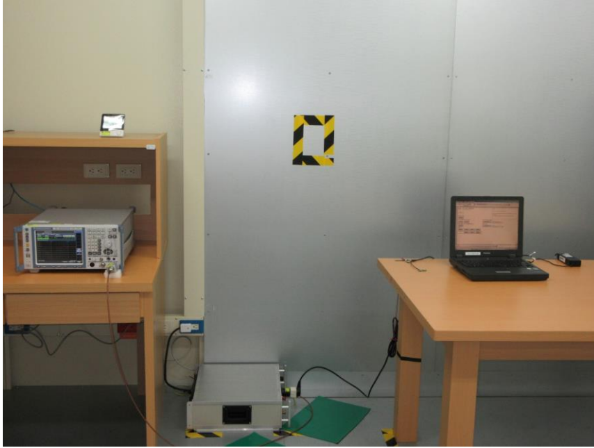
Photograph 9: Set-up for AC Mains (Front View)
