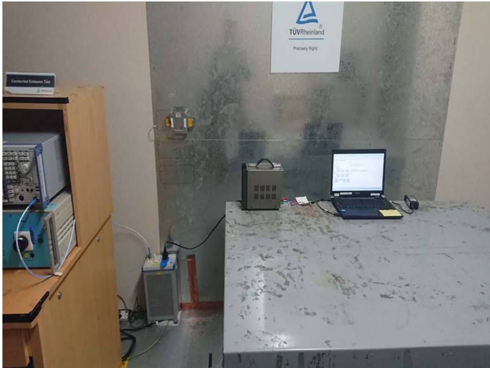
Photograph 8: Set-up for Mains Conducted testing (Back View)
