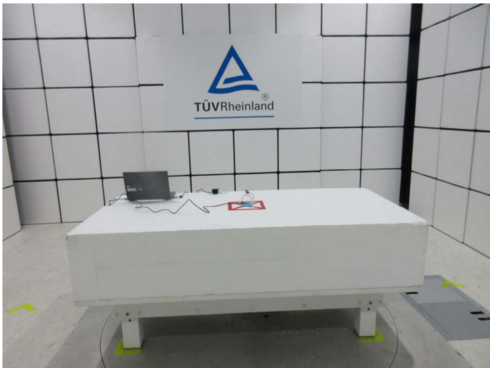
Photograph 1: Set-up for Spurious Emissions (Front View 1)
