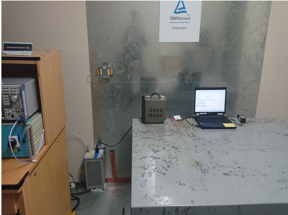
Photograph 8: Set-up for Mains Conducted testing (Back View)
