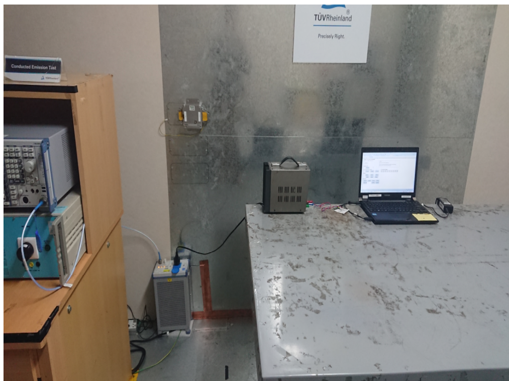
Photograph 7: Set-up for Mains Conducted testing (Front View)
