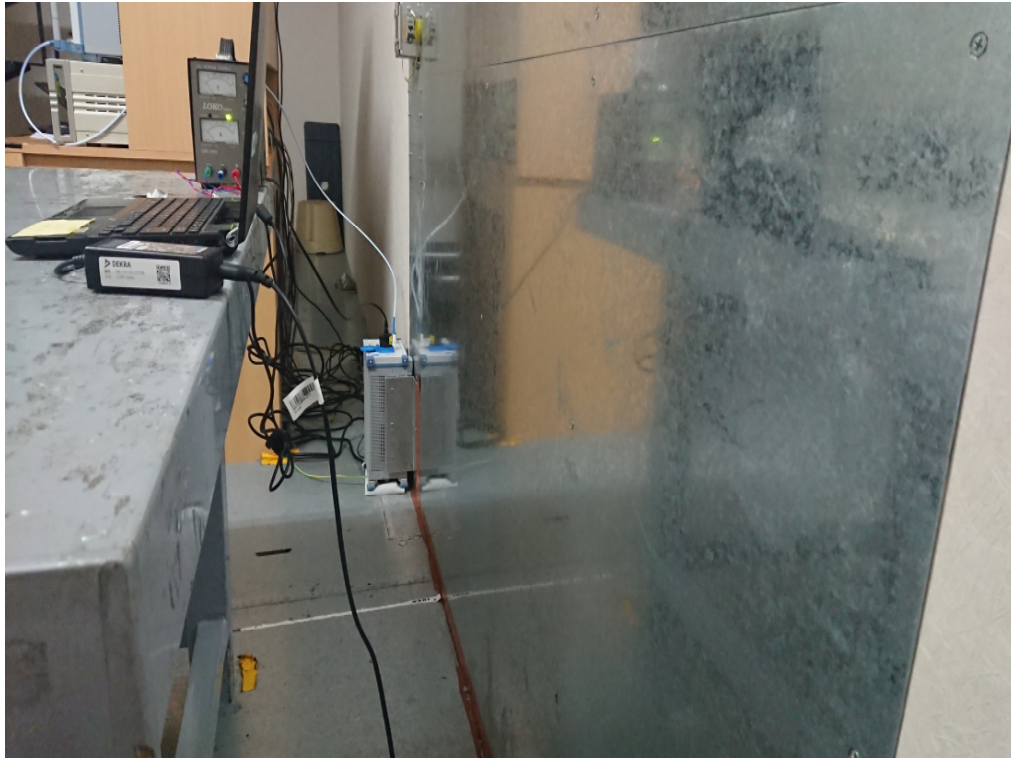
Photograph 8: Set-up for Mains Conducted testing (Back View)
