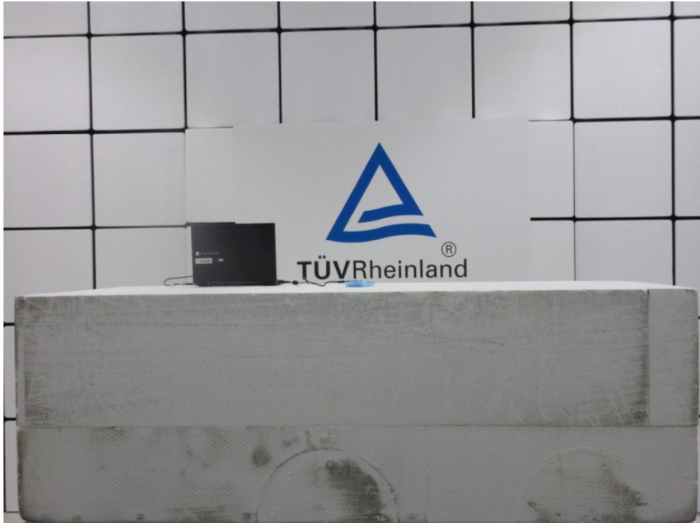
Photograph 3: Set-up for Spurious Emissions (Back View 1)
