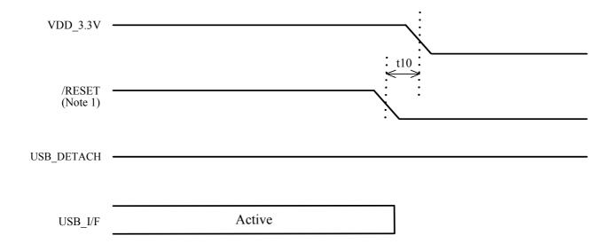
Timing Diagram for Power Down Sequence
