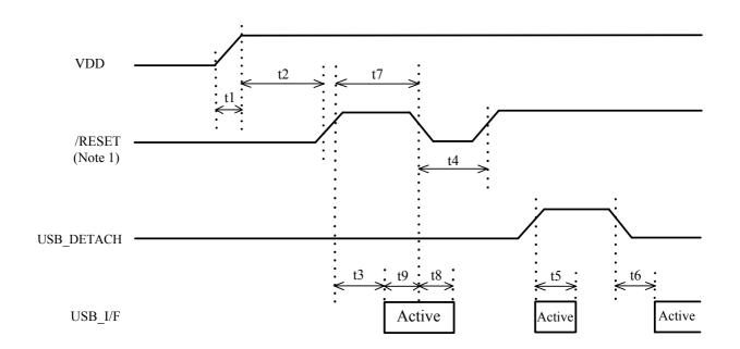
Timing Diagram for Power Up Sequence
