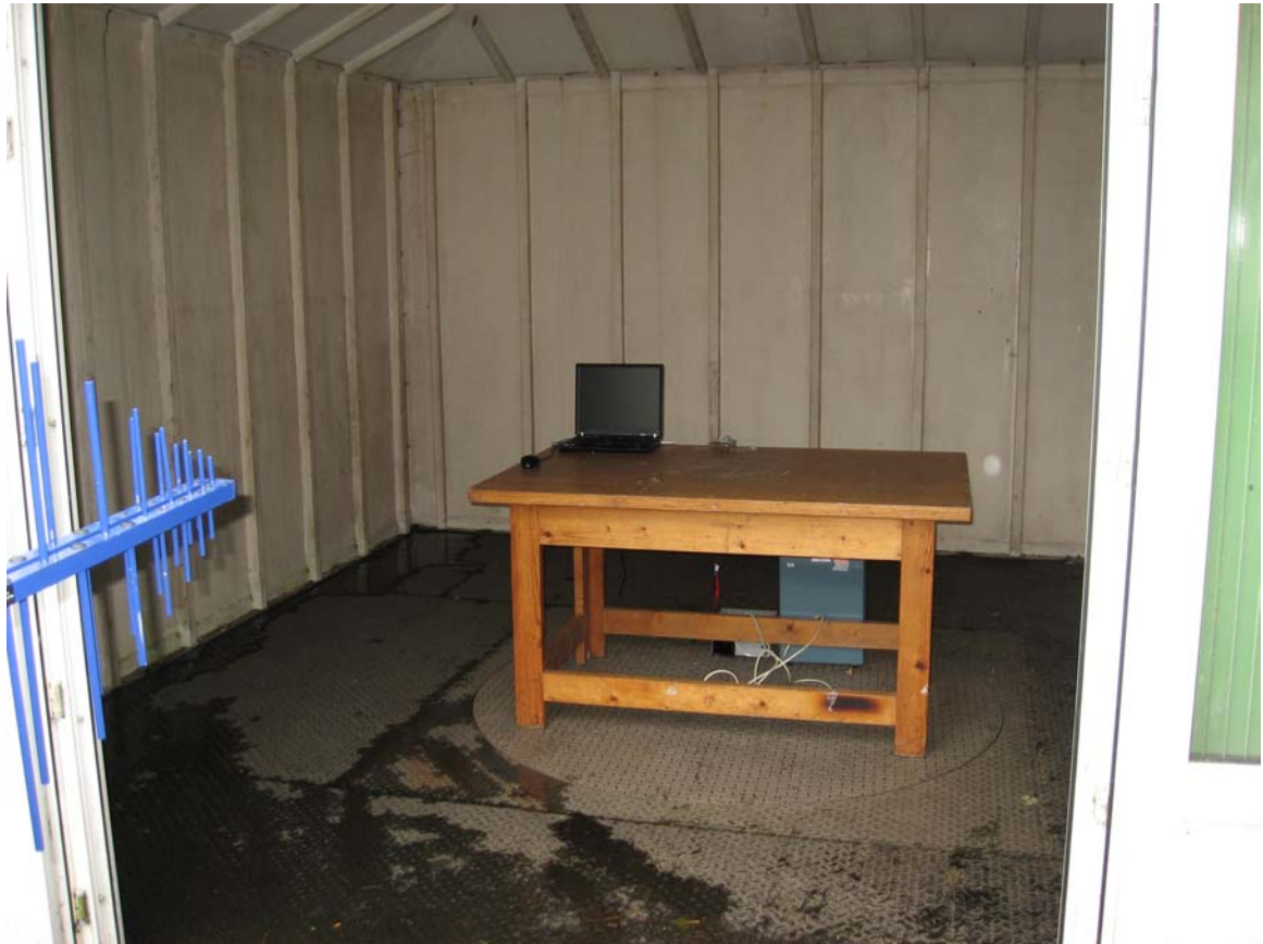
Photograph 1: Test setup radiated emissions - front
