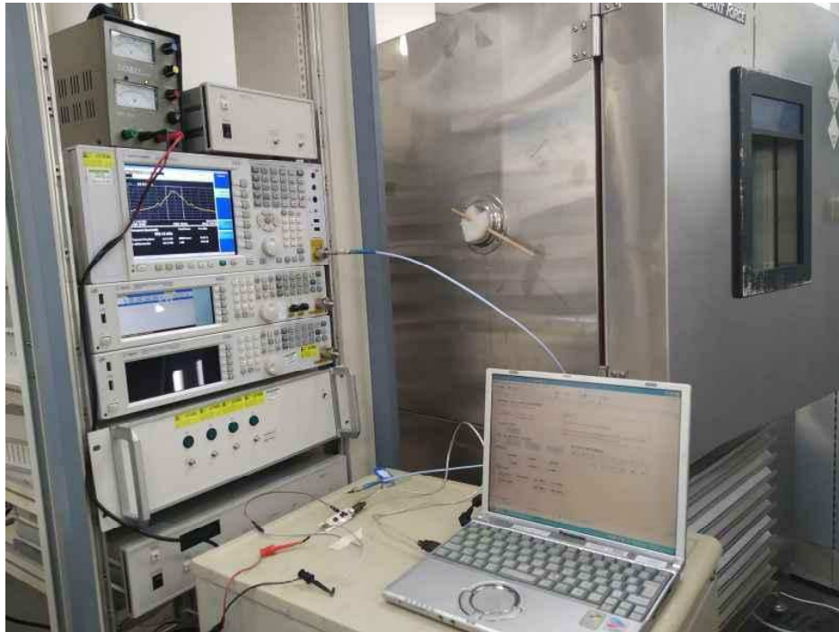
Photograph 8: Set-up for Conducted testing
