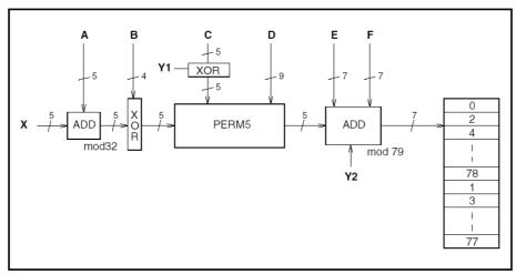
Due to the above flow, 32 nops are made into 5 ways. Then, the sign of the sign nead 160 is formed. The remainder that is worked out by dividing with 79 is assigned to Hopping Channel.
