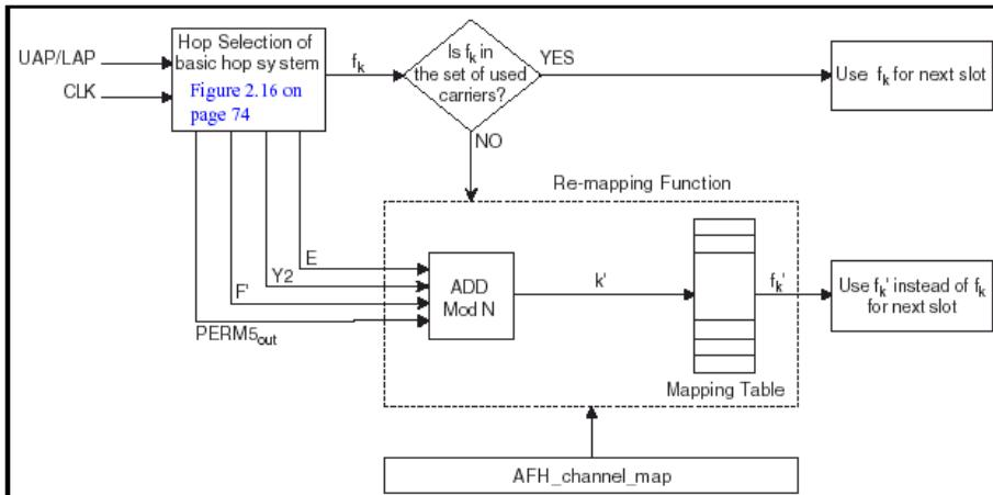
Also as the case of 79Hopping. Hopping Pattern uses the value that is worked out by dividing with the number of AFH-Channel's. Then, available Hopping becomes even as well as 79Hopping.
