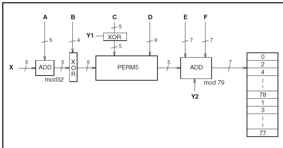
Due to the above flow, 32 hops are made into 5 ways. Then, the sign or the sign head 160 is formed. The remainder that is worked out by dividing with 79 is assigned to Hopping Channel.
