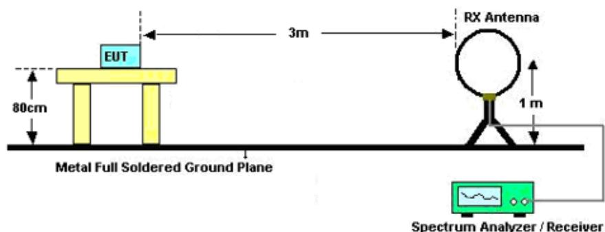
For radiated emissions from 30MHz to 1GHz
