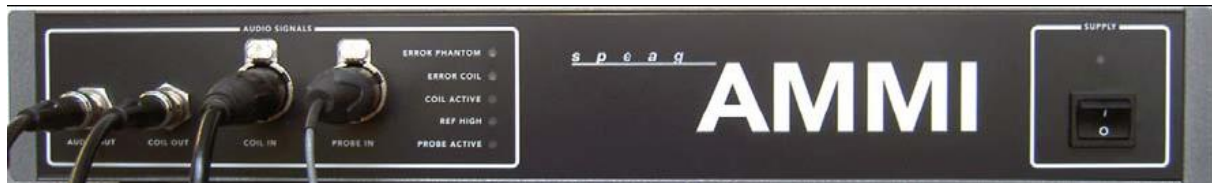
Figure 5.3 AMMI front panel
