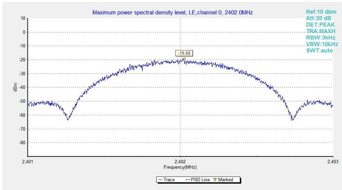
Fig.25. Maximum Power Spectral Density Level Function: GFSK, 2402 MHz
