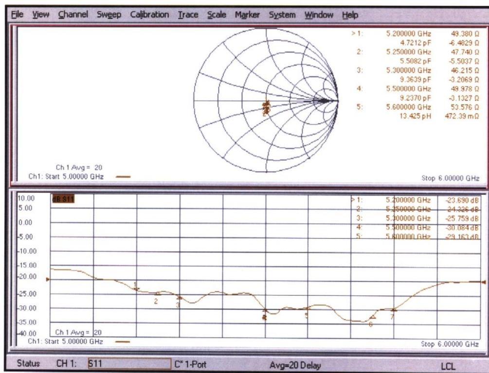
**Impedance Measurement Plot for Head TSL (5300, 5500, 5600, 5750, 5800 MHz)**
