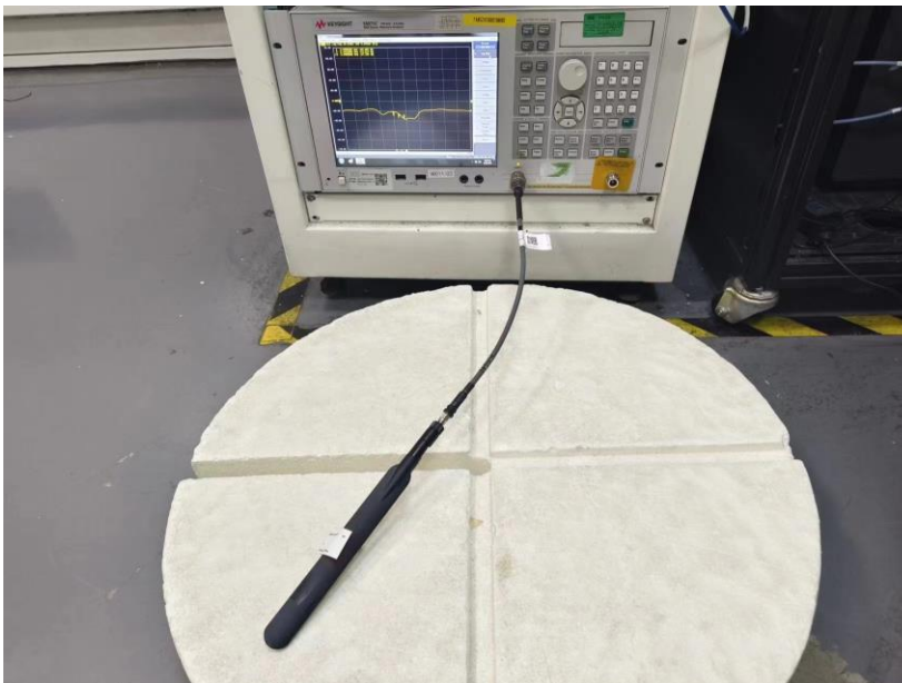
Free Space Impedance Setup - ANEPRA5-CAG03-EH
