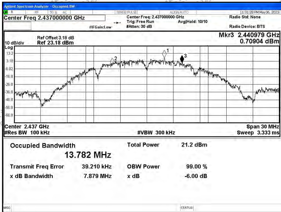
-6dB Bandwidth NVNT b 2437MHz Ant1
