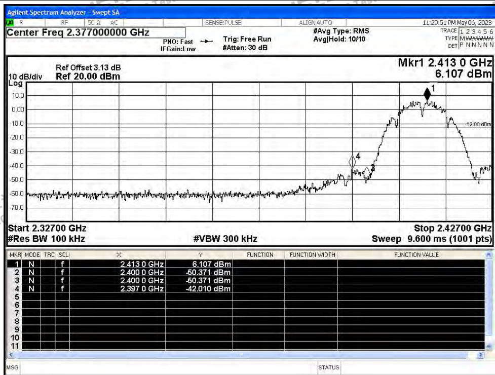
Band Edge NVNT b 2412MHz Ant1 Emission
