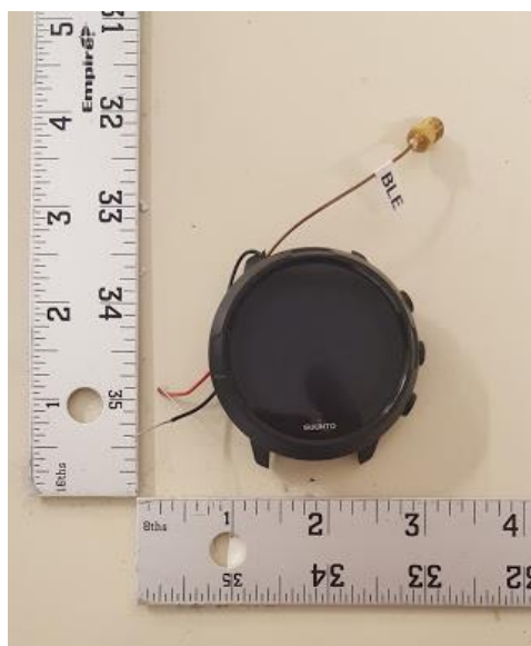
Figure B3. Conducted DUT
