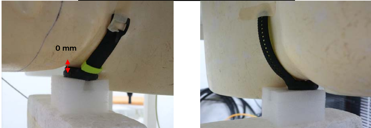
Fig.3 Back side of EUT to flat phantom
