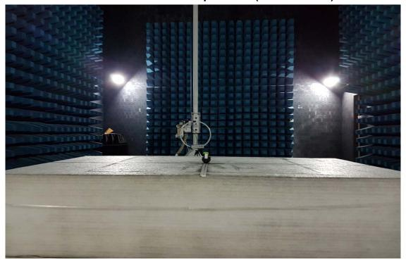
Radiated Emission Set up Photos (Below 1GHz)
