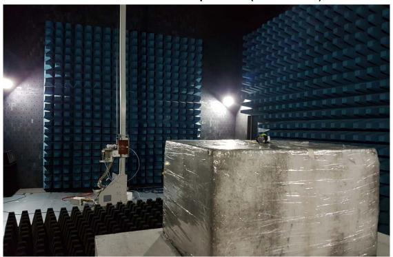
Radiated Emission Set up Photos (Front View)
