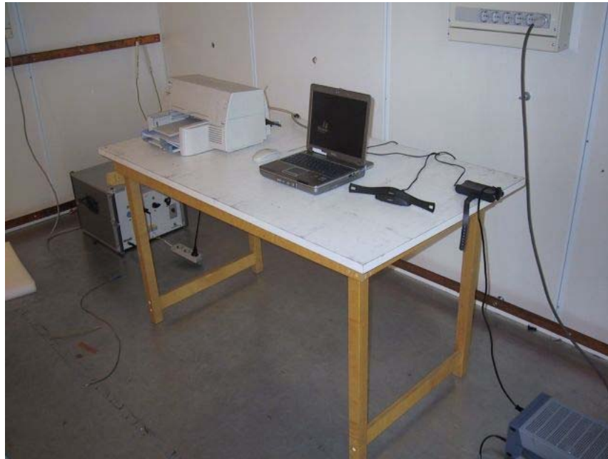
Picture 3: Conducted emission measurement setup
