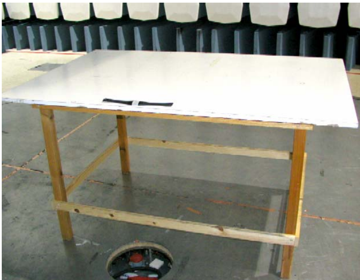
Photograph 2. Radiated emissions test setup
