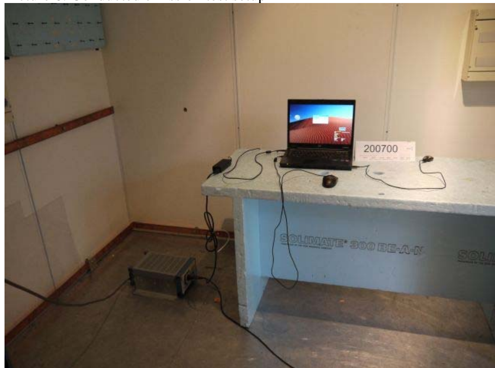
Picture 6: Conducted emission test setup
