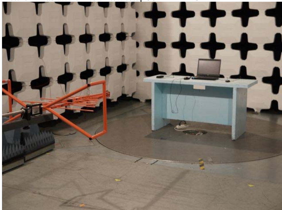
Picture 4: Radiated emission test setup 30 MHz – 1 GHz
