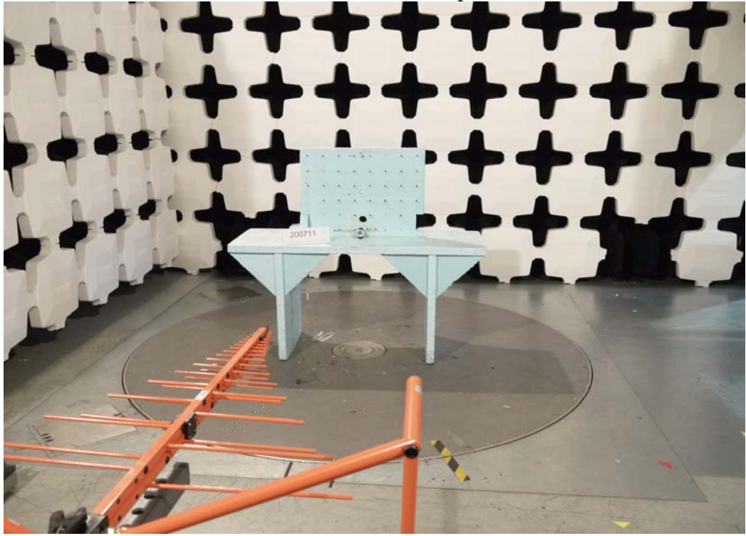
Picture 1: Transmitter Radiated emission test setup 30 MHz – 1 GHz
