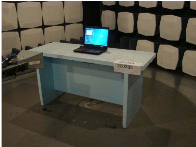
Picture 6: Transmitter Radiated emission test setup 3 GHz – 18 GHz.
