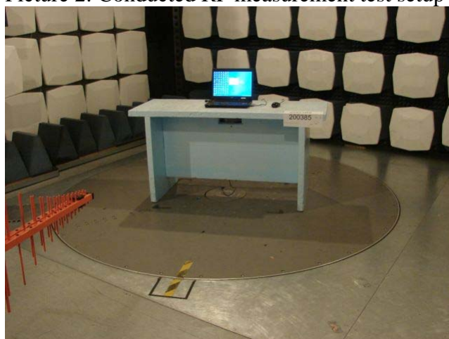
Picture 3: Receiver Radiated emission test setup <1 GHz
