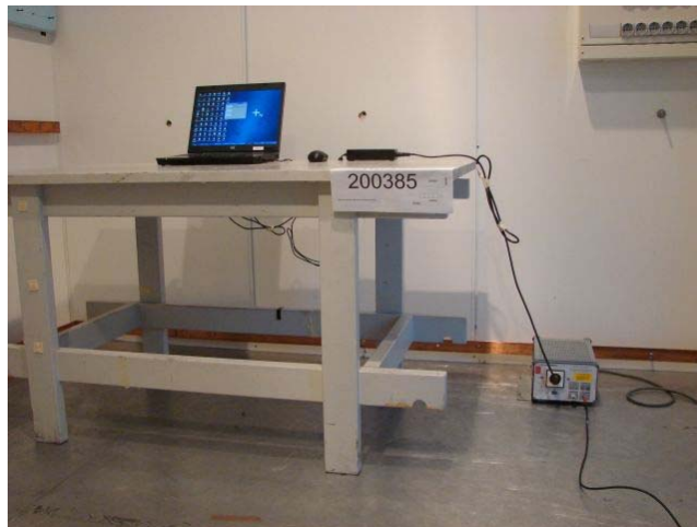
Picture 1: Conducted emission measurement test setup
