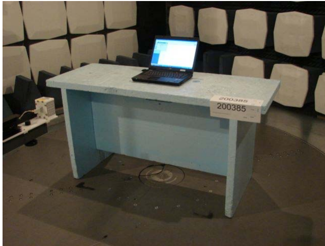
Picture 7: Transmitter Radiated emission test setup 18 GHz – 26 GHz.
