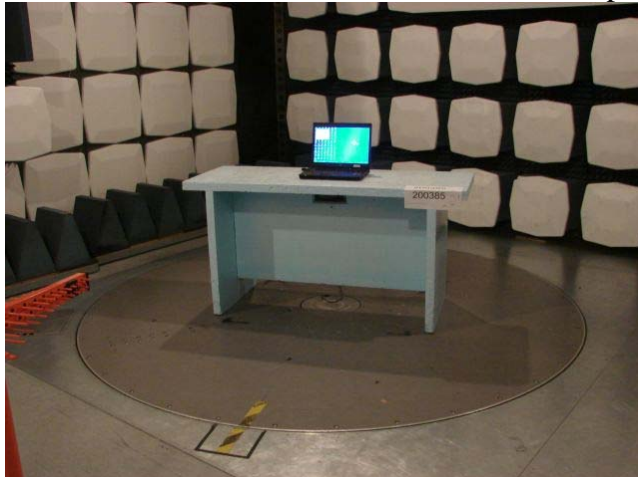
Picture 5: Transmitter Radiated emission test setup <3 GHz
