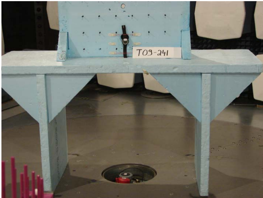
Picture 1: Radiated emission test setup <1GHz
