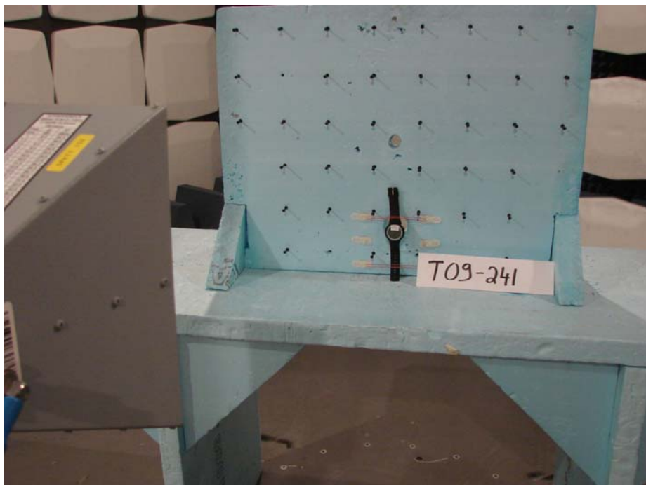
Picture 2: Radiated emission test setup 1 GHz – 18 GHz
