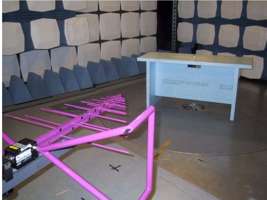
Picture 1: Spurious emission and field strength measurement setup
