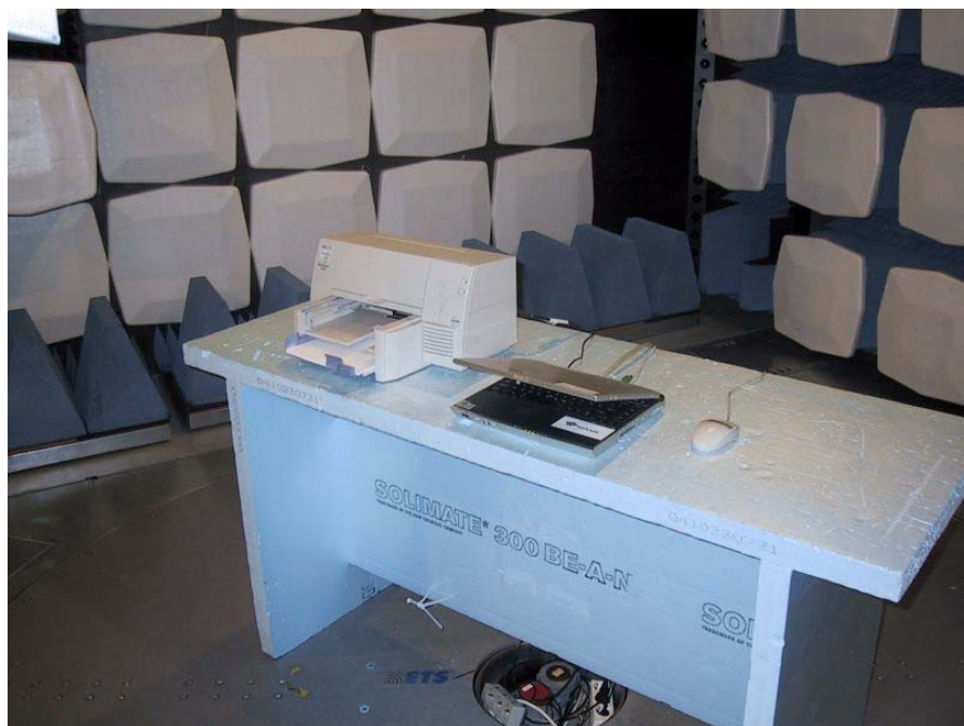
Picture 2: Radiated emission measurement setup
