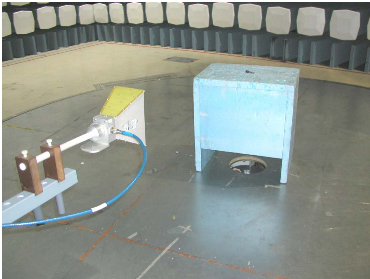
Photograph 2. Radiated emissions test setup
