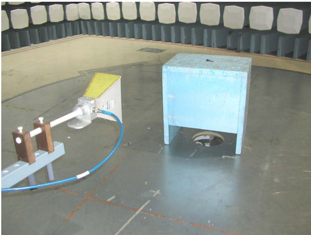
Photograph 2. Radiated emissions test setup
