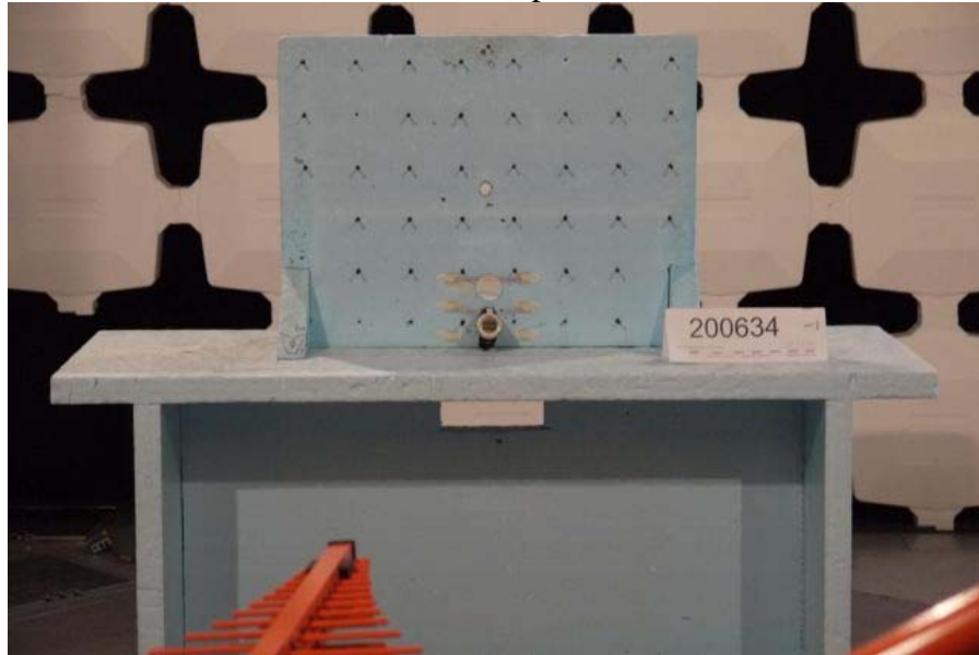
Picture 1: Radiated emission test setup 30 MHz – 1 GHz
