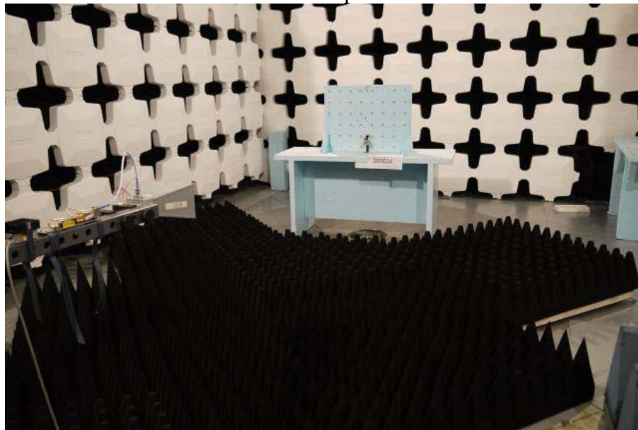
Picture 2: Radiated emission test setup 1 GHz – 16 GHz
