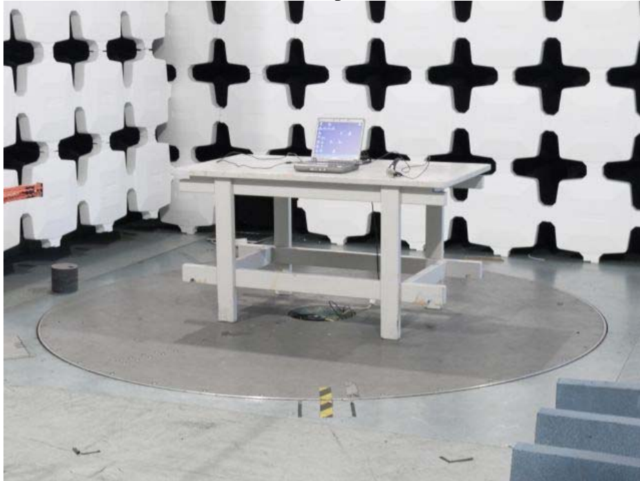
Picture 3: Radiated emission test setup 30 MHz – 1 GHz
