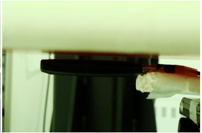
USB Cable Plug-in for USB Configuration 2 (Horizontal Down with Phantom 5 mm Gap)
