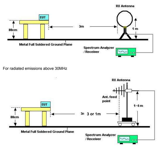
Above 10 GHz shall be extrapolated to the specified distance using an extrapolation factor of 20 dB/decade form 3m to 1m.
