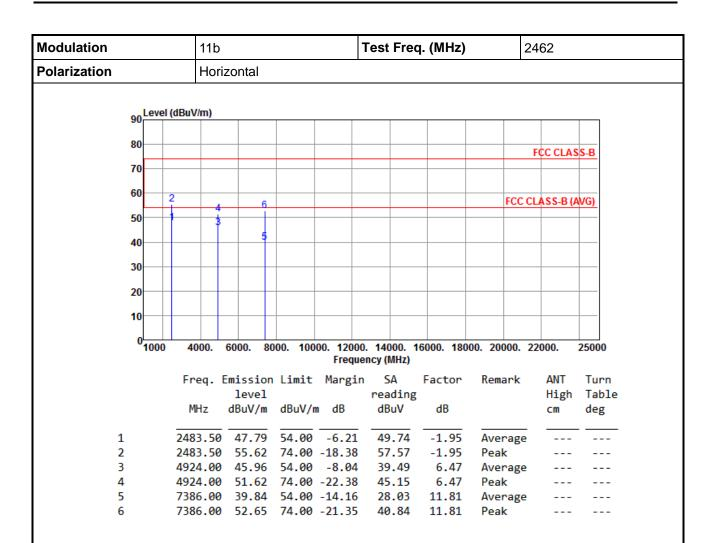
Note 1: Emission Level (dBuV/m) = SA Reading (dBuV/m) + Factor\* (dB)
